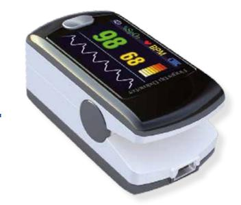
Portable device useful to detect the SpO2 quantity (amount of oxygenated hemoglobin in the blood and the heart rate through a non-invasive way.
